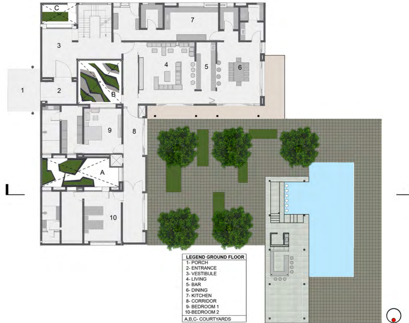
↑ Ground Floor Plan.
